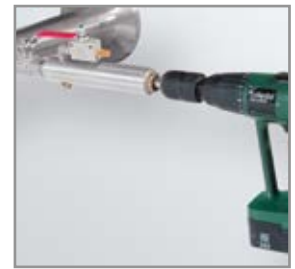
Drill under pressure with the PMH Drill
