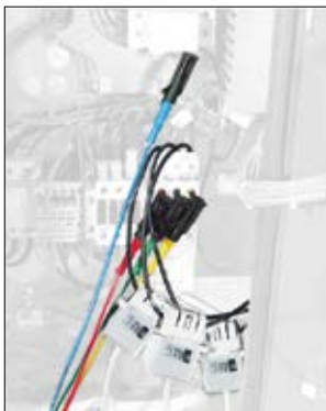
Magnetic voltage measuring tips electrically isolated
